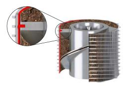
Fibers are caught in the patented profile groove of the auger, where they function as a brush. Metallic rubbing between the auger and the wedge wire screen is avoided by this brush.
